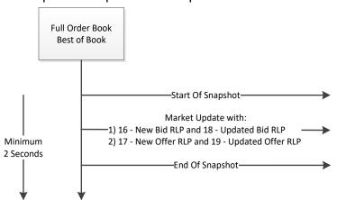
Both **Start Of Snapshot** (2101) and **End Of Snapshot** (2102) messages contain the last *Market Data Sequence Number* (MDSN) of the last real-time message taken into account by the snapshot (see <u>Sequence Numbers</u> and <u>Snapshot Sequence behaviour</u> for explanations on the MDSN). This last MDSN has been sent on each channel speed.
